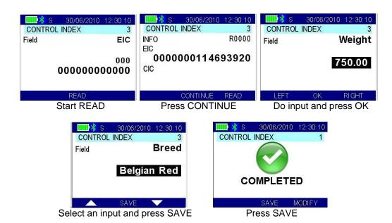
After having answered all the questions, press SAVE to write the input data into the current reading session file or press MODIFY to re-edit and correct the input data.
