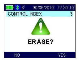
If the *Erase* function is confirmed, the device removes the selected data-set from the current control-file.
