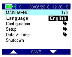
**Input via multiple-choice:** highlight the configuration field to be edited (left picture above) and press SELECT. The chosen field becomes bold (right picture above). At this point, press UP/DOWN to scroll along the predefined allowed values. Confirm the new value by pressing SAVE.
