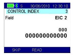
In the case the field repetition number is greater than needed, press SKIP to finish the field.
